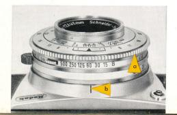
Note: the resistance between 1/30 and 1/15 sec serves as a warning that for photographs taken at 1/15 or B, the camera should be mounted on a tripod to avoid camera shake.
